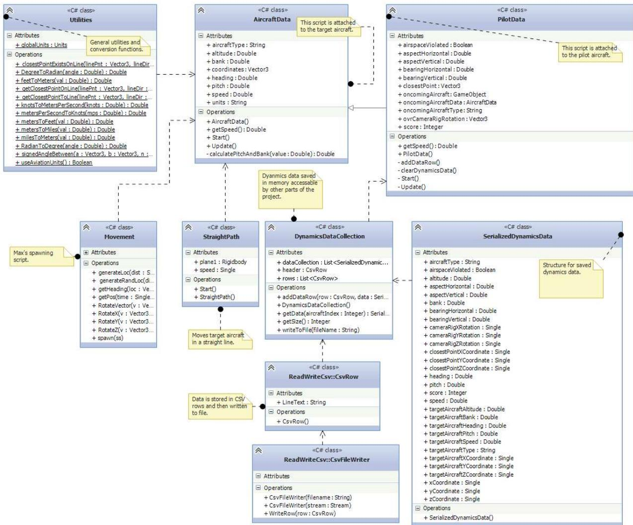
The AircraftData and PilotData scripts are attached to the target aircraft and pilot aircraft respectively. These scripts calculate the dynamics data. The StraightPath script is used by AircraftData in order to cause the target aircraft to move along a straight path.
